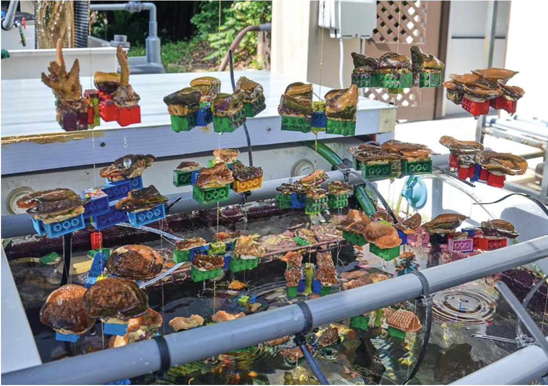
Figure 1.8.2: LEGO bricks used as substrate for coral reef restoration project, photo courtesy National University of Singapore
