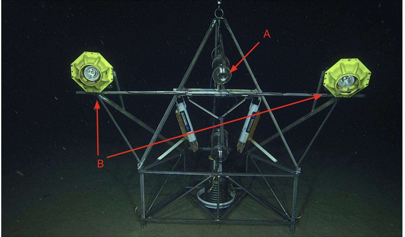
Fig. 1: Time series camera mounted on tripod at Station M, an abyssal site off the coast of Central California. A) full frame camera responsible for photos used during this study, B) strobes used to illuminate the seafloor during photo capture.
