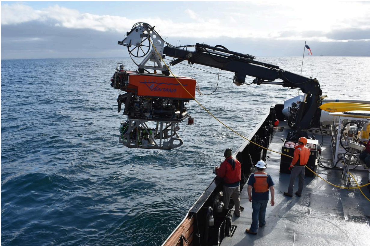
Figure 3: ROV Ventana held above the ocean surface to be inserted or removed from the water. The ROV's 2,300 meter umbilical cable allows the ROV to be controlled remotely from the ship control room. Real time video is placed on screens in the control room in order to ensure accuracy and precision of animal collection (photo by MBARI).
