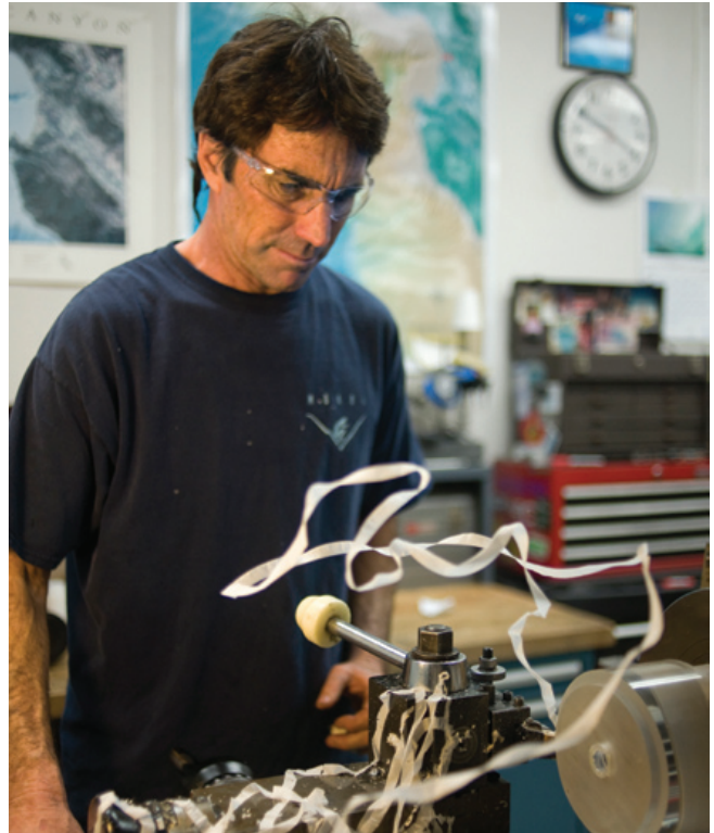
Figure 36: Mechanical Technician John Ferreira uses the lathe to conduct a materials test on acrylic that will be used in manufacturing equipment to be deployed in the ocean.
