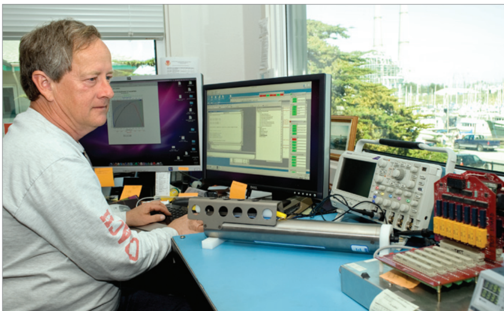
Figure 34: Software Engineer Rich Schramm programs a new instrument driver for the controller for MBARI’s OASIS 3 moorings. Every new instrument type requires the creation of a new driver to sample the instrument and log its data. OASIS 3 now has drivers to handle data from more than 30 oceanographic instrument types commonly used on MBARI oceanographic moorings.
