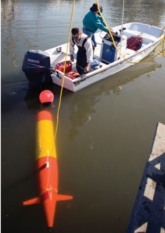
Figure 29: Thomas Hoover (front) and Chris Wahl launch the long range autonomous underwater vehicle, Tethys , during early field tests in Moss Landing Harbor.
