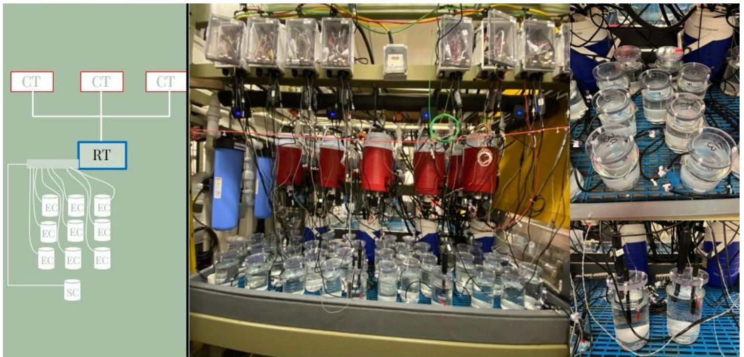
Figure 2: Diagram of upwelling system set up (left). Image of the complete lab set up with red conditioning tanks at the top, blue reservoir tanks at the bottom back portion of the water table, and the clear experimental tanks along with sensor tanks at front of the water table (center). Close-up images of 9 replicate ECs and examples of SCs with their corresponding sensor probes (right).
