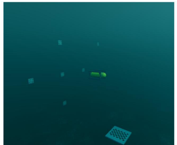
Fig. 6. Depiction of the replicated test tank Apriltag layout along with the ROV in the simulation
