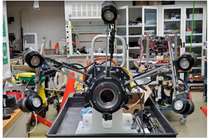
EyeRIS in the lab with the light array expanded. This is the benthic configuration, which eliminates one of the lights for better ground clearance.
